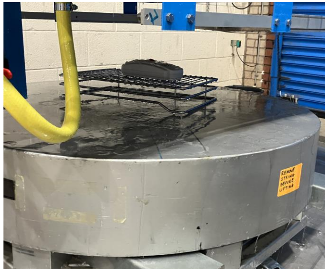
Specimen S6 orientation 1 Ingress Protection Test, IPX1
