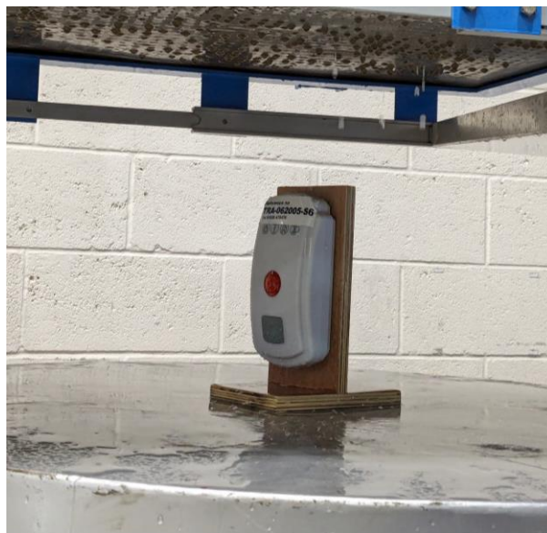
Specimen S6 orientation 2 Ingress Protection Test, IPX1
