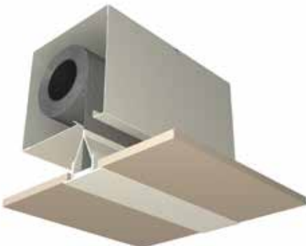
Reinforced Suspended ceiling with recessed shadow gap
